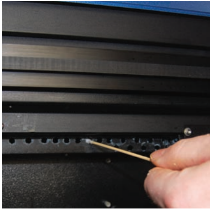
Figure 6: The upper exhaust inlets consist of a series of holes located just under the “X” rail. These holes tend to clog up with debris and must be cleaned regularly.
