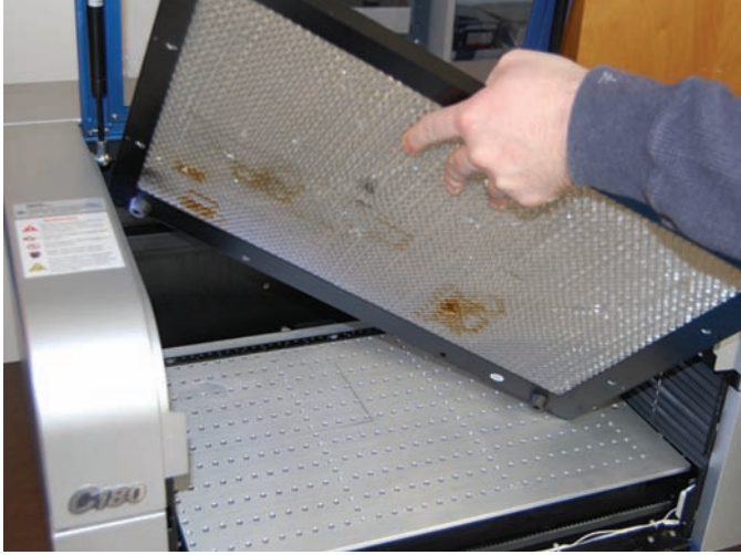
Figure 11: The honeycomb cutting tray can be installed by lowering the engraving table and joggling the grid table into place. It can also be bolted in place for very precise, multiple pass engraving.
