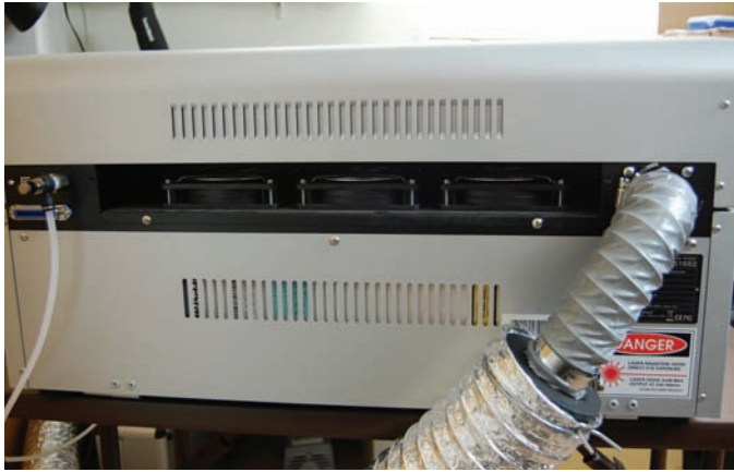
Figure 5: The LaserPro C180 is unusual in that it uses a 2" exhaust. Since all blowers I know of are either 3" or 4", the hose has to be converted.
