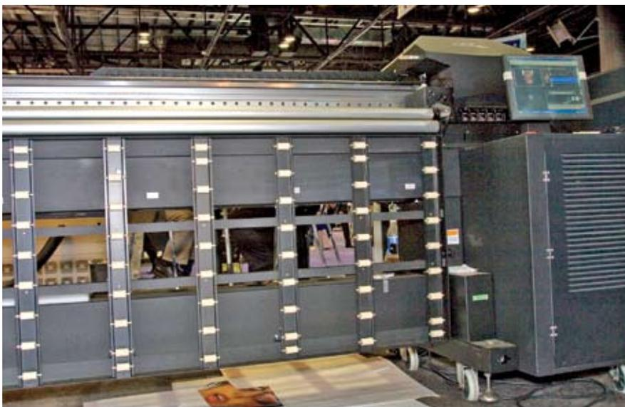
Fig. 4: Fold the roller tables against the printer when you're ready to switch from rigid to flexible media.
