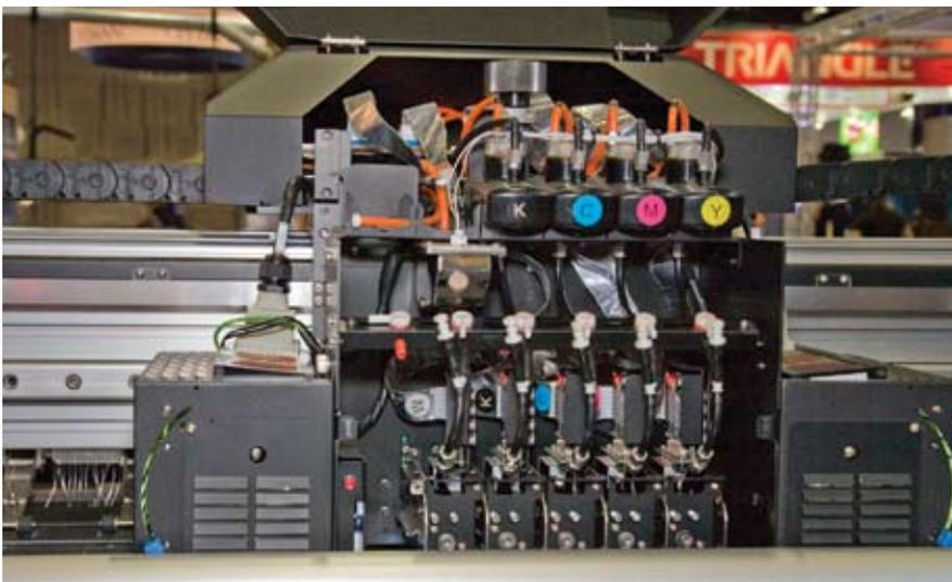
Fig. 1: A view of the StellarJET 183UVK's carriage mechanism. Notice the CMYK print heads. Options for this printer include light cyan, light magenta and white inks.
