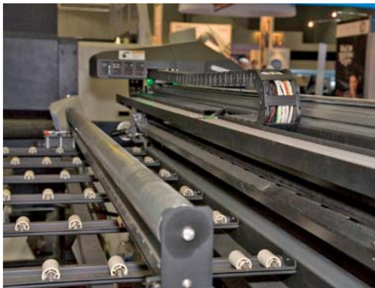
**Fig. 3:** This 183UVK table view shows the stout rollers and the media bar, all designed to keep rigid media aligned.
