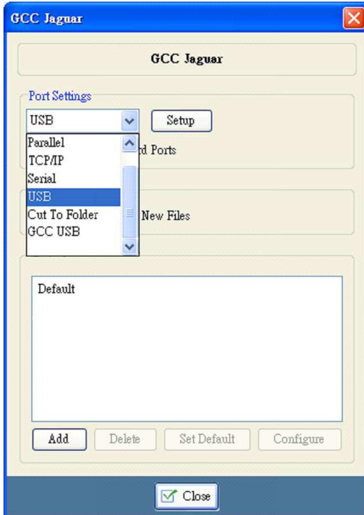
Step 5. Select "Add Image" to input your image to the working area (the cutting line of this file must be set as "CutContour") and select "GCC Jaguar" in "Cutter" at the lower left corner.
