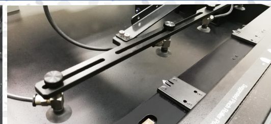
Suction cap for automated sheets feeding process
