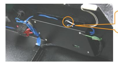
LCD Display Screen's Contrast Adjustment Wheel
