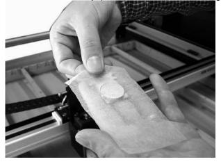
8) Allow the mirror to dry before re-installing it.
