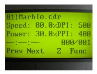
The main work page is the page that the LaserPro X500 SERIES will default to upon startup and will be the "home base" for when navigating through the various functions of the control panel. This will be the page that is displayed when you are processing your jobs. This page contains specific job information such as the current job's name, Speed, Power, PPI, DPI, processing / remaining times, and jobs loaded.
