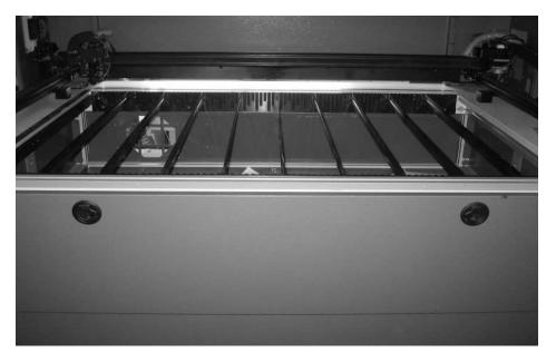
• Place the Honeycomb Table or Aluminum Grid Cutting Table over the arranged Supporting Cutting Bars.
