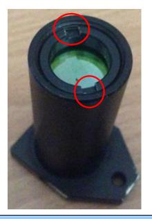
Fit the Focal Lens Removing Tool here
