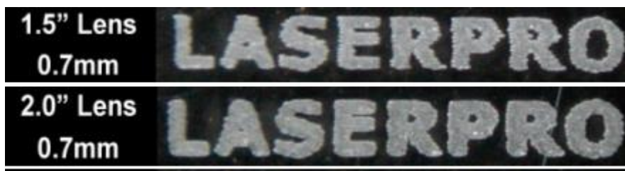
Cutting edges achieved with the different lenses
