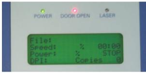
Figure 4: The red light on the control panel alerts the user if the door is open.
